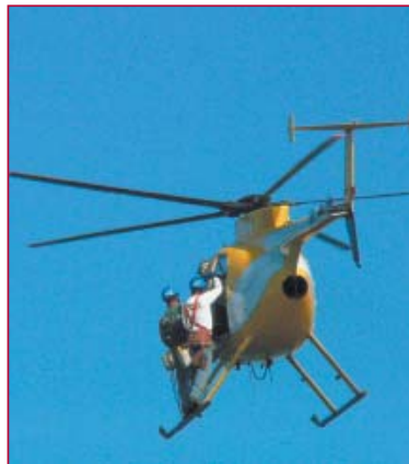
The crew rides to the next pole on the landing skid of the helicopter traveling at 40 miles per hour.
